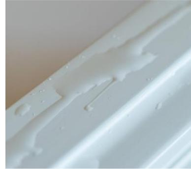
**FAIL** – If the surface fails the wet-ability test (i.e. the water beads into multiple droplets) the surface must be cleaned again.
