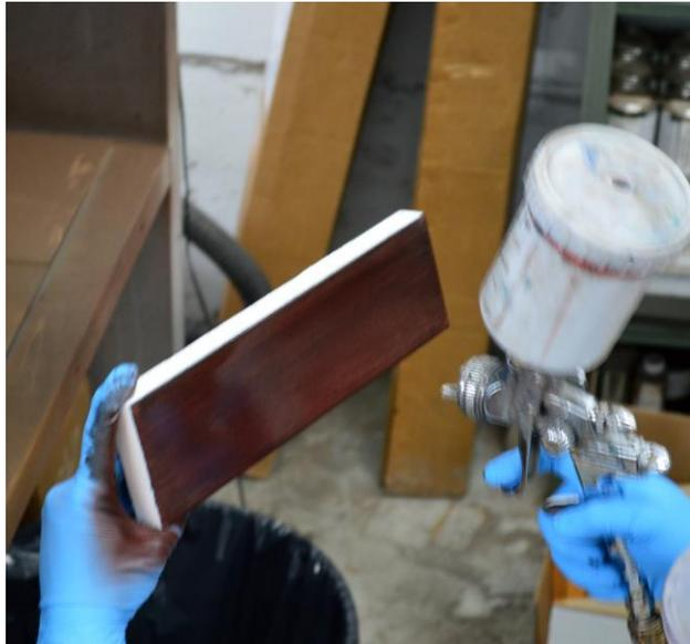
Stain Top Coat should be filtered through a cone filter strainer or mesh filter before pouring the coating into the spray equipment.
